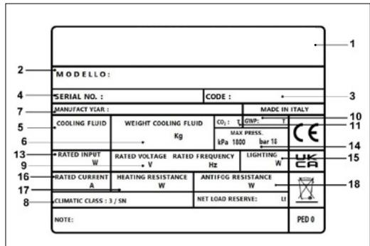
A serial plate is affixed behind the equipment, stating all its identification and characteristic data:
