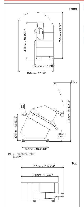
Electric Supply voltage: 600110 (DTRSC) 220-240 V/1N ph/50 Hz Electrical power max.: 0.37 kW **Total Watts:** 0.37 kW Capacity: Performance (up to): 400 kg\hr Key Information: External dimensions, Width: 246 mm External dimensions, 557 mm Depth: External dimensions, Height: 466 mm **Shipping weight:** 21 kg
