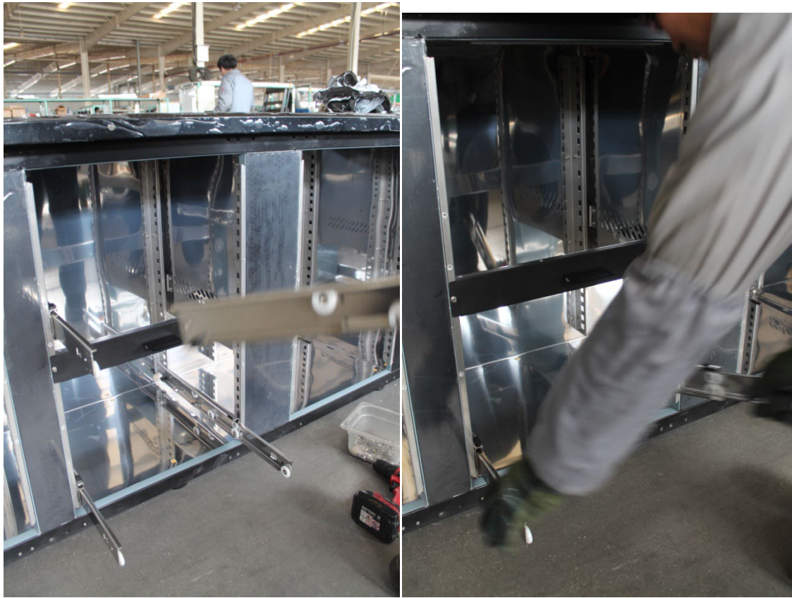
2.remove the guide from the support
