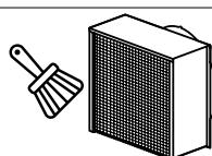
After every cleaning operation it is necessary to rinse with warm water and dry the unit with a soft and clean cloth. Clean the condenser, after having removed the cover grid, with a dry paint brush (do not use iron brushes) or a vacuum cleaner, removing all dust and possible deposits on the fins.
